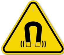
Keep the device at least 1 meter away from magnetic sources and any devices sensitive to magnetic fields.
